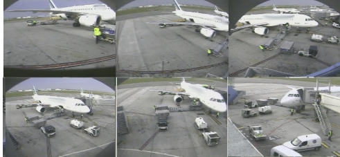
Fig. 1. Videos are captured from six cameras and tracking is fused to get ground plane data.
